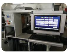
The Nano Paste is ergonomically and safely designed; all operations are performed from a single position in front of the dispenser.
