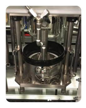
Once mounted on the Nano Paste, all base colours' cans will remain sealed thanks to dedicated follower press-plates, which will prevent air and dirt from contaminating the inks.
